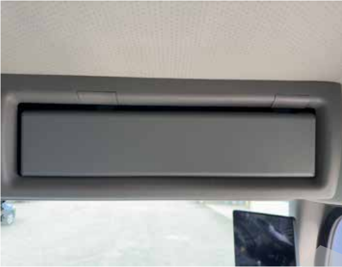
Cut out netting and install close-out panel
