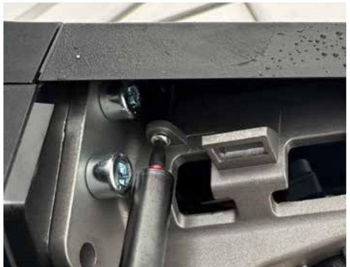
Using the corresponding fastener set, install upper cover to the Main Bracket/Arm
