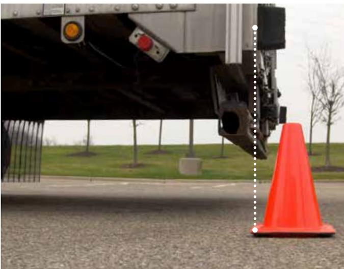
Before doing so, first place cones at the end of the trailer on both the driver and passenger sides of the truck ...
