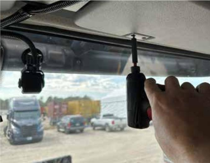
Uninstall point screws from upper console to install the Class V monitor bracket
