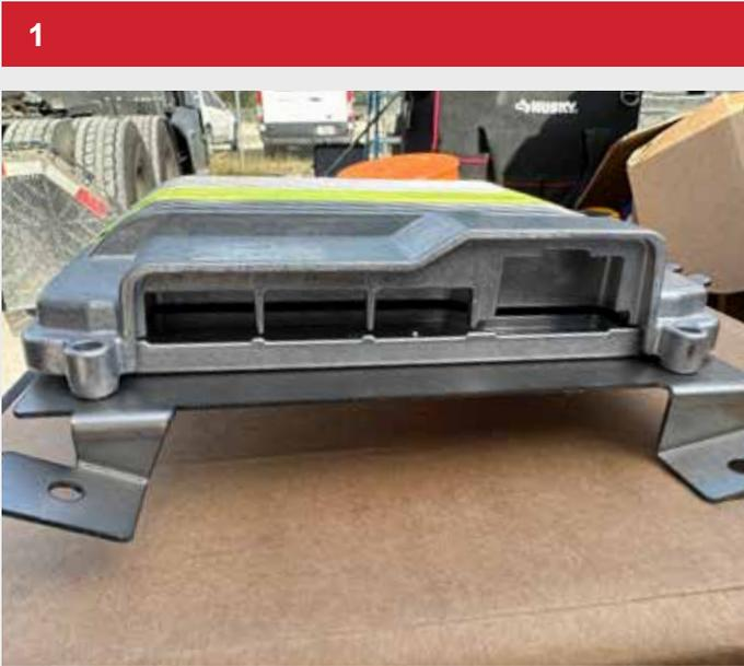
Using the corresponding screw set, attach the DVR module to its bracket
