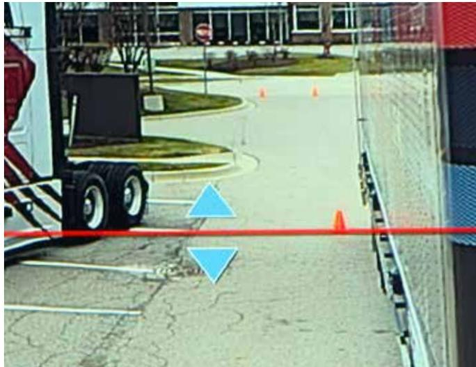
Match the red line on the monitor with the cone at the end of the trailer on the Driver Side using the Dial Knob ... when it's aligned, push the Controller Knob ...
