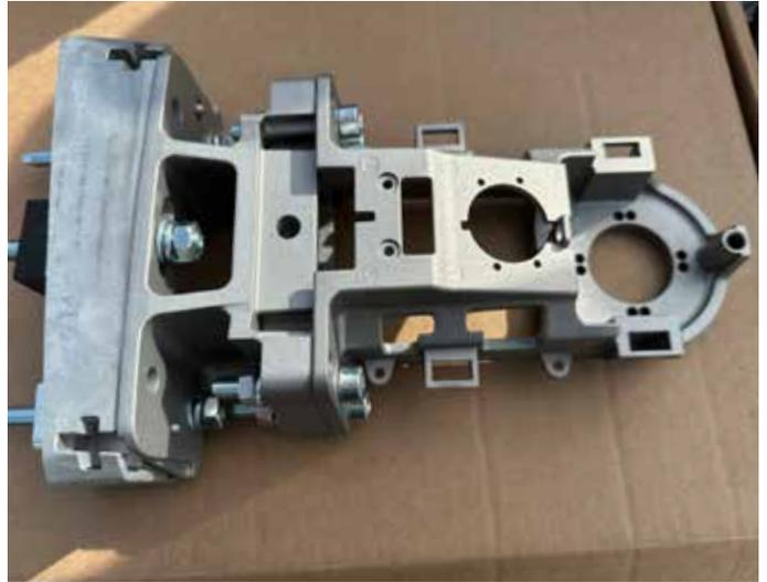
The passenger side camera/arm assembly consists of four components: (1) Backplate Bracket (interior side) (2) Interface Bracket (exterior side) (3) Extension Bracket (4) Main Bracket/Arm
