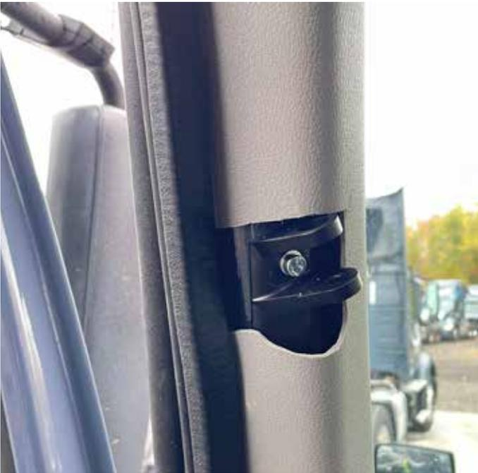
Using the location and size of the A-pillar interface bracket for reference, cut a rectangular hole in the relating side (driver/passenger) A-pillar cover removed during pre-installation. With the relating monitor (driver/passenger side) in hand, thread the cables through the A-pillar cover; make connections to the MirrorEye® harness connector and camera cable. Relating images depict process to finished bracket/A-pillar assembly
