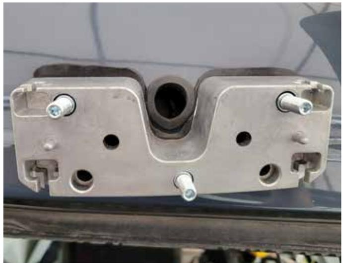
Place relating exterior gasket and center-hole grommet in place, then align the Interface Bracket by with the M8 two-way screw set
