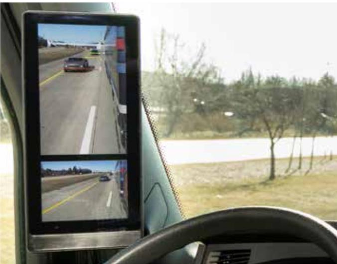
For the driver side camera view make sure that the horizon is parallel to the top of the monitor screen. Align the inside edge of the camera view to be parallel with the fairing
