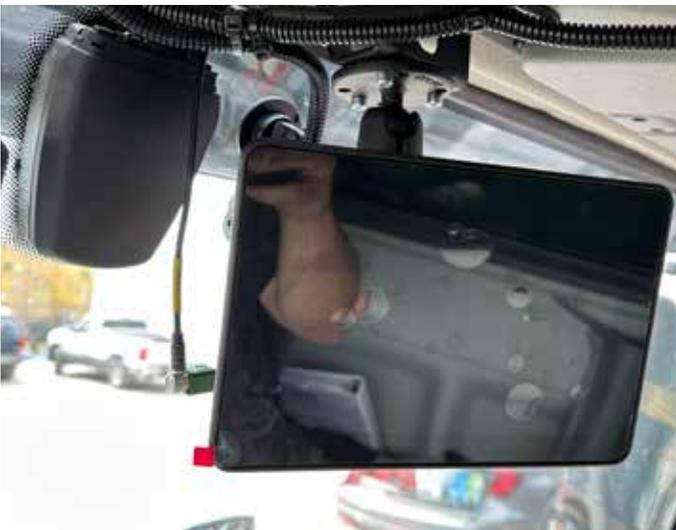
Assemble the central bracket and RAM® base, adjusting with an impact driver. Install monitor with the screws that are indicated in the kit to assemble the bracket; USE SHORT SCREWS with red Loctite® visible
