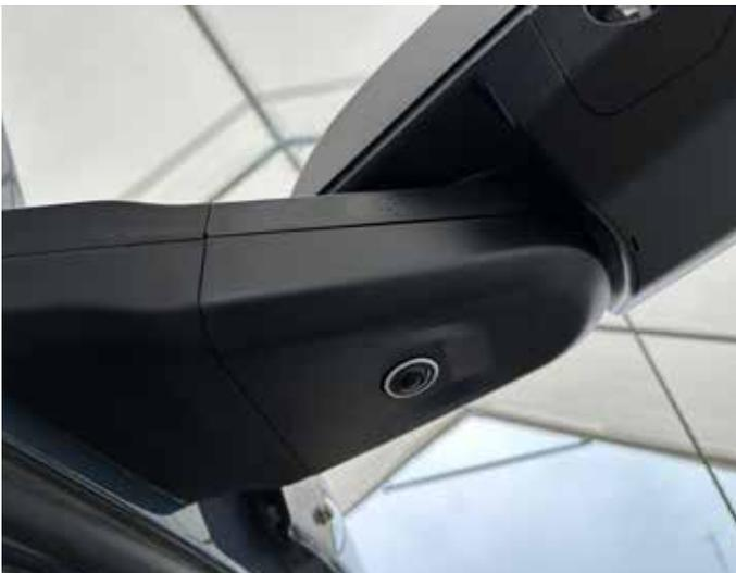
Install passenger side camera wing to Main Bracket/Arm (completed passenger side arm/camera, assembly depicted)
