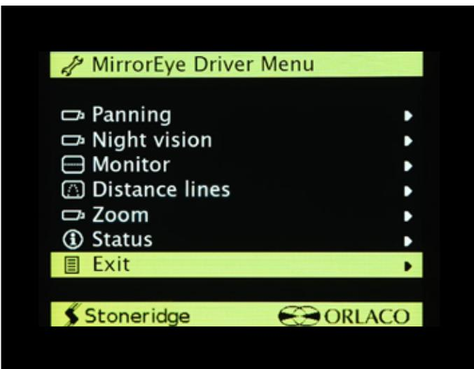
Using the controller's dial knob, scroll down to the Exit selection, and **long-push the Driver Side Manual Panning button and Controller Knob simultaneously** ... this will bring access to advanced settings ...
