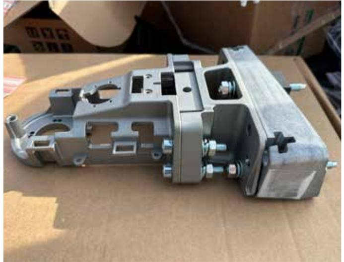
The driver side camera/arm assembly consists of four components: (1) Backplate Bracket (interior side) (2) Interface Bracket (exterior side) (3) Extension Bracket (4) Main Bracket/Arm
