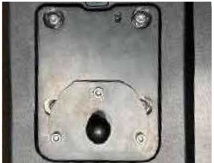
Install RAM<sup>®</sup> base to the monitor with relating kit set screws (NOTE: Red Loctite<sup>®</sup> should be on screws; passenger-side monitor is 15")
