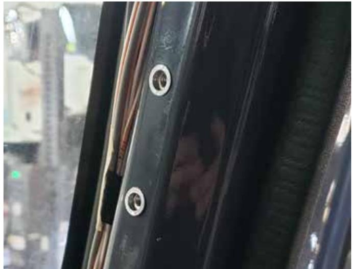
Use the monitor bracket as a template to measure hole locations on the passenger side pillar. Make two (2) holes with 10mm drill bit and insert the Riv-Nuts using Riv-Nut puller tool
