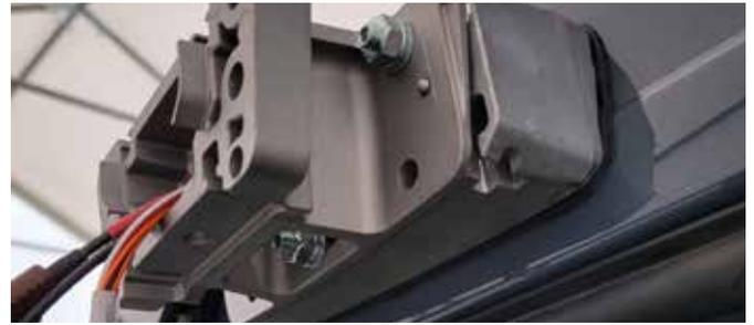
Ensure the relating driver side harness and coax cables is routed through cable pass-through hole and mounted brackets
