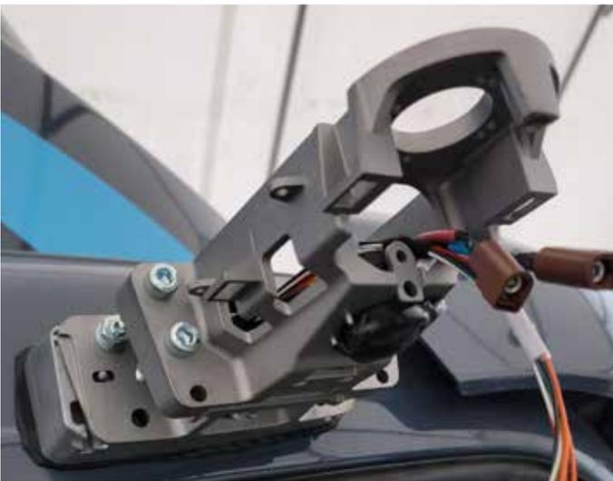
Attach the Main Bracket/Arm with corresponding screw set and route affiliated cables/connections
