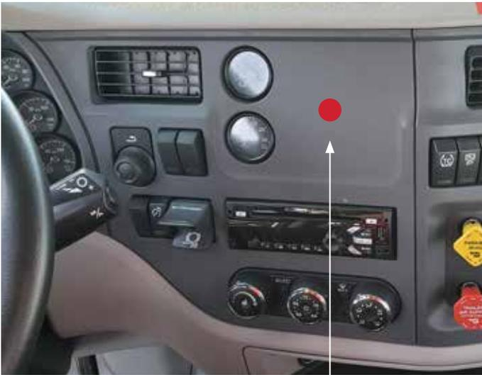
The MirrorEye® controller/joystick is installed on the dash panel to the right of the driver (see image above). On CNG-equipped PACCAR trucks, the relating CNG gauge will need to be relocated to the position depicted above (red circle)
