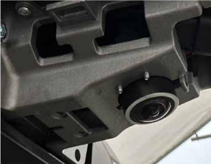
Install the Class V (blind spot) camera in the center position of the Main Bracket/Arm (as depicted), while being careful to not scratch/damage the lens
