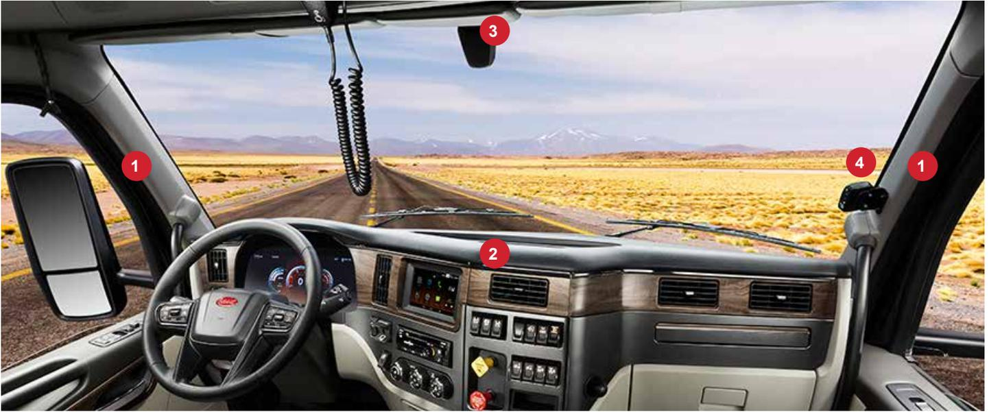
Prior to the installation of MirrorEye® system components, the A-pillar covers (1) center dash panel (2) should be removed and the headliner (3) should be adjusted to allow for access at the center windshield (4) XXX blind spot indicator removal XXXX.
