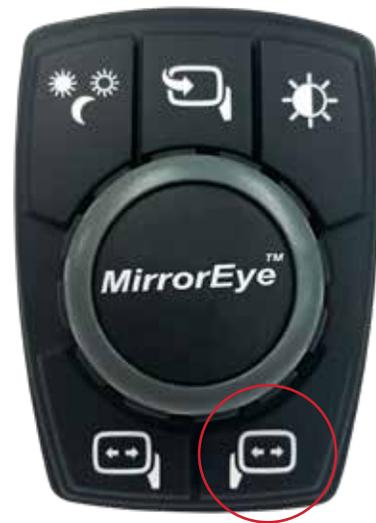
To match Passenger Side distance lines with those of the driver side, push and hold the lower-right button on the MirrorEye® Controller ...
