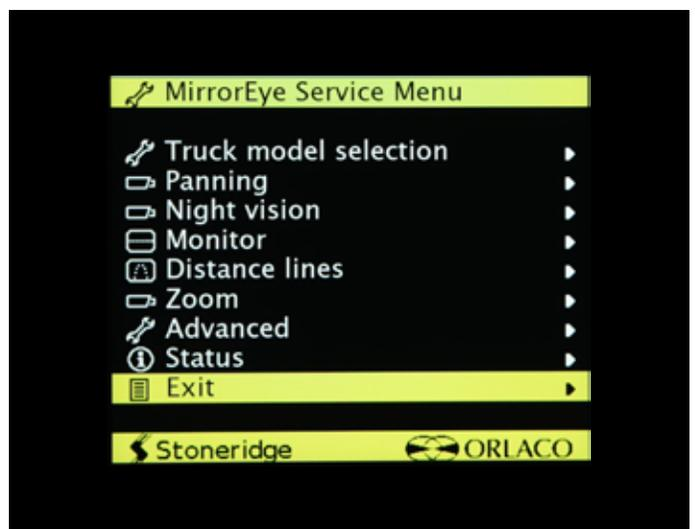
To exit the Service Menu, scroll down to Exit and press the Controller Knob again ...
