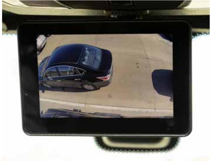
The Class V camera should show as parallel to the truck's body and should be positioned to maximize the outward view
