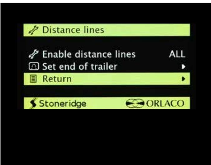
To exit Distance Lines in the Service Menu, dial-scroll to Return and push on the Controller Knob ...
