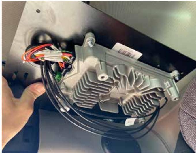
The crossed slitted opening to be by the top of the ECU Assy, so it is not visible after the ECU Assy is completed mounted
