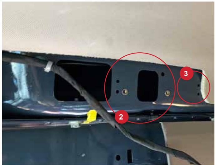
Once the door frame's trim (1) is uninstalled with its door's light, the existing M4 mounting features that are used to attach the door's ambient lamp, will be used to mount the ECU's Bracket (2) and another two existing holes at the right (3) to be used to apply M6 rivets and bolts. In total 4 fixing points for the ECU Bracket.
