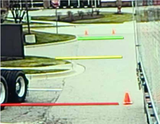
At the time of installation, the vehicle's distance lines **must** be calibrated in the MirrorEye® system ...
