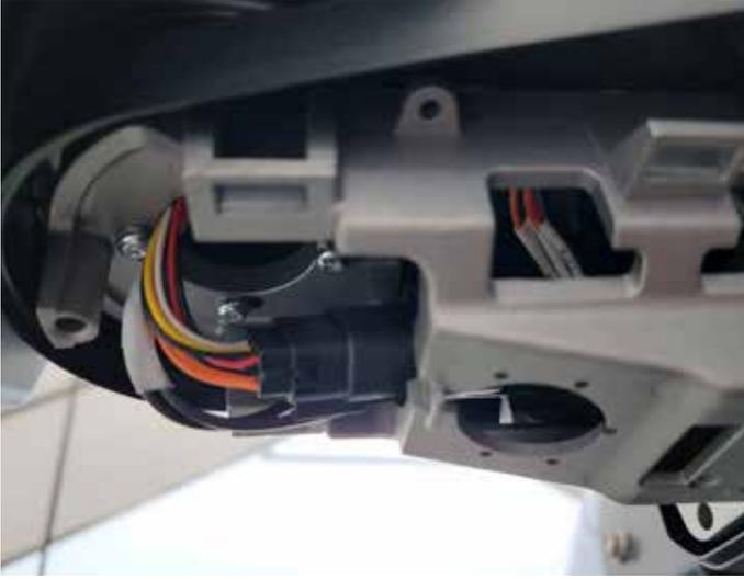
Before affixing lower cover, ensure the assembly of the Main Bracket/Arm (depicted) and all connections are secure and unkinked
