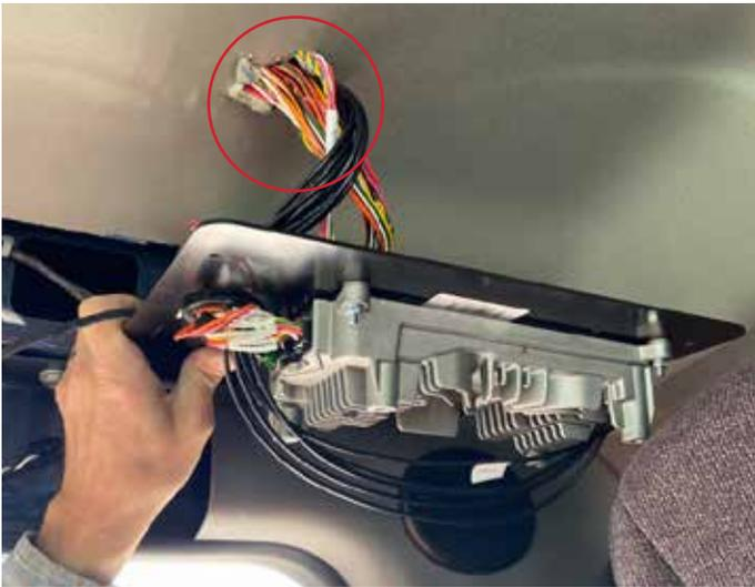
The ECU Assy is positioned to mark up the upper head-trim location's hole to be created for the harness and coax cables to pass through. After the crossed slits are done, the harness and cables get through it to continue and complete the routing from the ECU.
