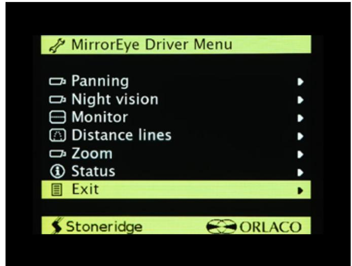
Using the controller's Dial Knob, scroll down to the Exit selection, then **push and hold the Driver Side Manual Panning button and Controller Knob simultaneously** ... this will bring access to advanced settings ...
