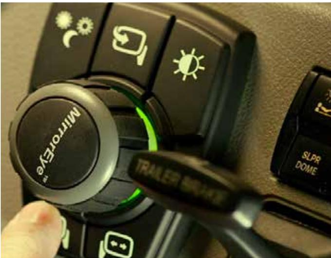
**NOTE:** Take note of the light indicators — if green lights do not turn on, there is a misconnection within the system. If the mis-connect cannot be identified, make contact with Stoneridge representative(s)
