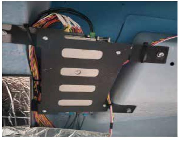
ECU Fit in location with very little room to spare. Designed holes lined up correctly which allowed for a smooth installation.
