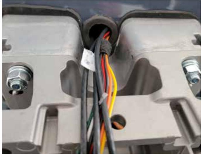
Route the relating passenger side harness and coax cables relating to Wing Camera and Class V (blind spot) camera through cable pass-through hole
