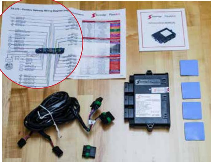
Assemble the connectors as depicted in the provided FA 470 schematic – note that the center shroud is for an additional connector (blind). Each module connector is numbered (CN 1,2,3).
