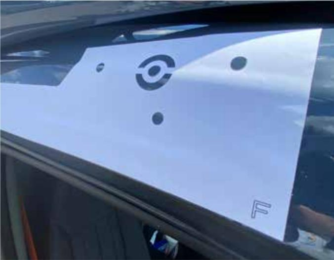
Use template provided to identify mounting M8 mounting hole locations (3), and center-located 1" cable pass-through hole
