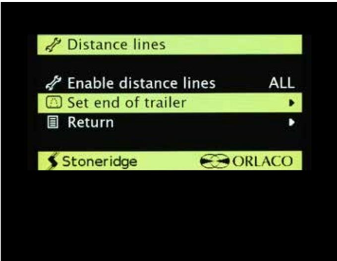
Back in the cab, dial-scroll to the “Set End of Trailer” selection and push the Controller Knob ...
