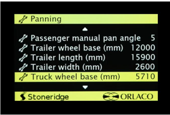
To adjust the **Wheelbase**, scroll to the selection in the Panning menu and press the Controller Knob ...
