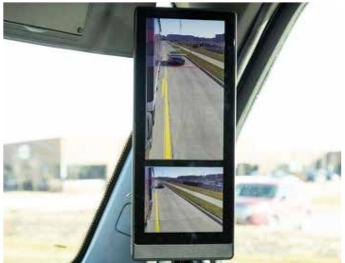
Repeat the previous step (3) on the passenger side ensuring a similar field of view in both the driver side and passenger side monitors
