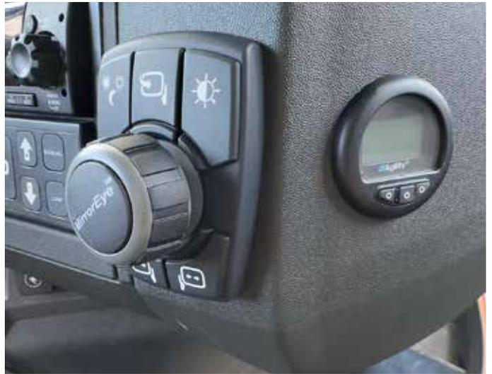
Installed controller (including relocation of CNG gauge)
