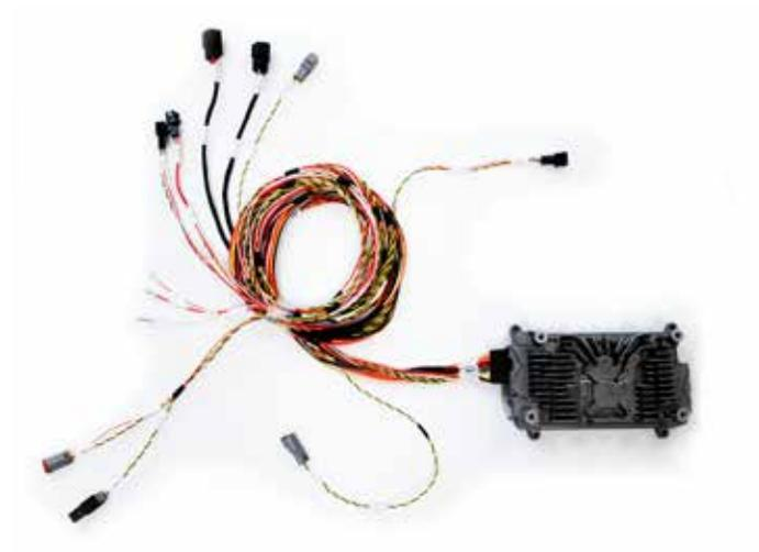
Please take every measure to avoid kinking of wires when working with/handling the main MirrorEye® ECU wiring harness (Y-harness). Kinked lines can lead to communications interruptions between components and the system network.
