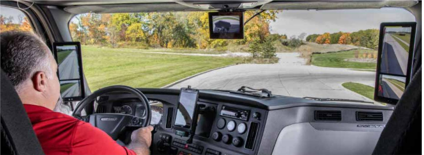
Confirm the system powers up properly and that all monitors are showing the correct feed from their respective cameras
