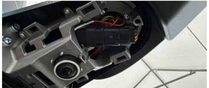
Using the corresponding fastener set, install upper and lower covers to the Main Bracket/Arm
