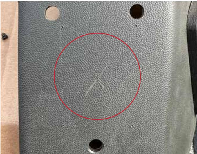
Create the cut-out hole using a 2 1/8" tool at the location depicted.
