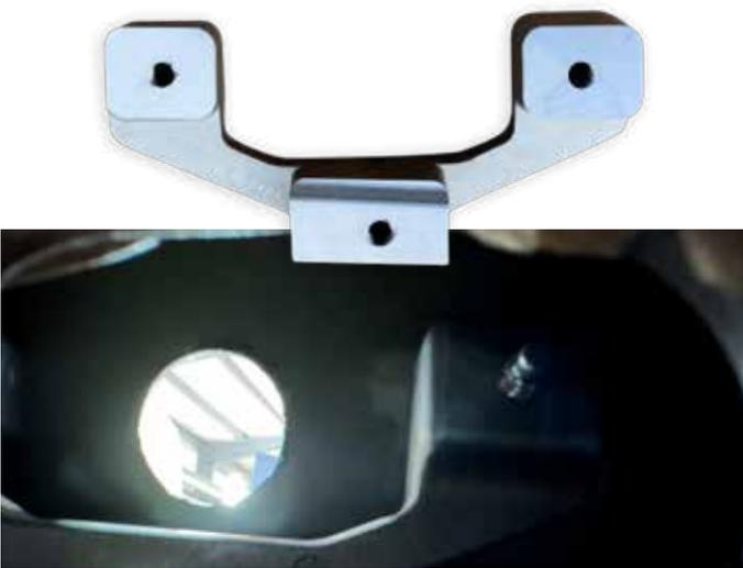
Identify Backplate Bracket, then affix from interior of driver side (depicted) with corresponding M8 two-way screw set
