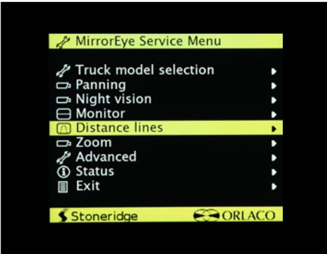
On the MirrorEye® Service Menu, dial-scroll to Distance Lines, then press the Controller Knob ...
