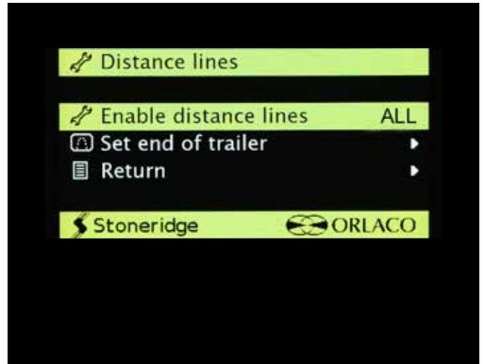
MirrorEye® installation technicians need to set the End of Trailer – or EOT – distance to calibrate the vehicle's distance lines ...
