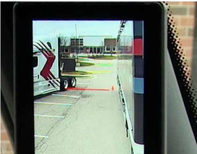
Once set, the correct driver-side distance lines are adjusted and displayed on the monitor ...
